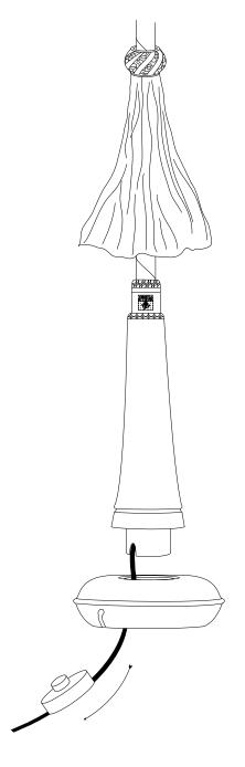
1. Pass the electrical wire through the cast iron base.
