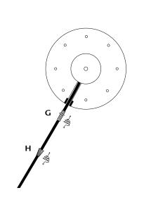
3. linsert the wire within the groove and fix it to the base with elements **G** and **H**.
