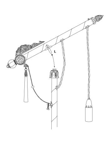
5. Place the rod in horizontal position inserting the peg  ${\bf L}$  into the stand.
