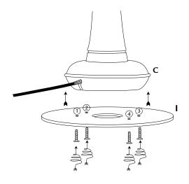
4. Fix the metal disk I to the base **C** with the 4 screws.
