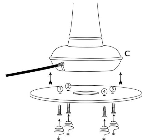
4. Fix the metal disk I to the base C with the 4 screws.
