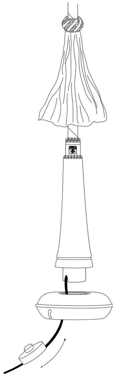
1. Pass the electrical wire through the cast iron base.
