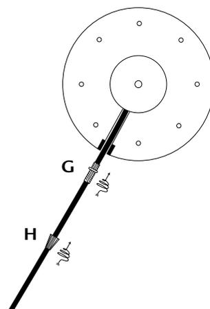
3. Insert the wire within the groove and fix it to the base with elements G and H.
